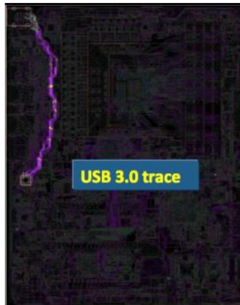
**Figure 3. PCB trace between a USB 3.0 port and the physical host controller on a motherboard, highlighted in purple**
