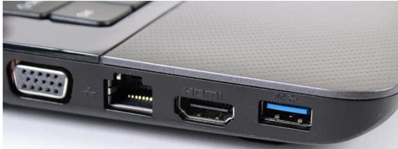
**Figure 1. The signature pantone blue USB 3.0 port on a laptop**
