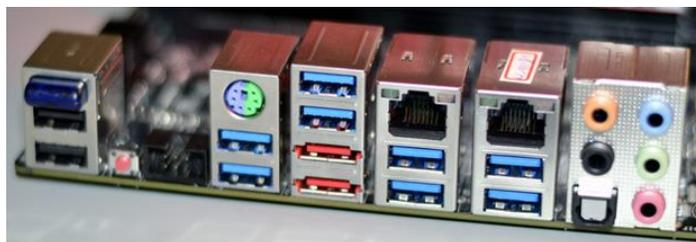
**Figure 4. A motherboard with 8 USB 3.0 ports**
